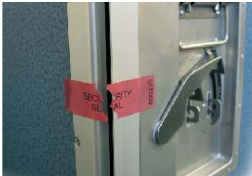
Easy breakage of seal when door is opened leaving effective removal tabs
